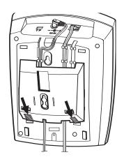
7. Align the base's keyhole slots with the mounting screws, and slide the base downward to secure it.
